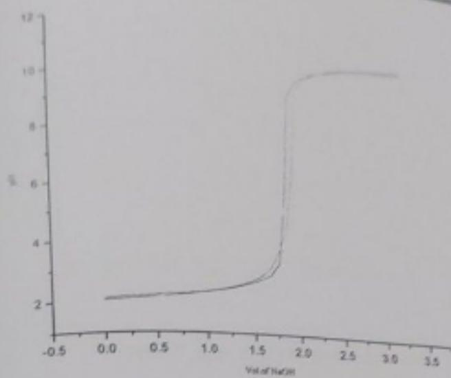
Graph 1.5 pH metric titration curve for Co (II) + Nicotinic Acid (1:1 ratio)
