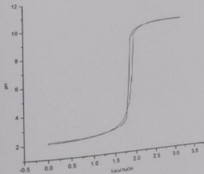
Graph 1.2 pH metric titration curve for Ni(II) + Nicotinic Acid (1:1 ratio)
