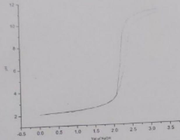
Graph 4.1 Potentiometric titration curve for Cu (II) + PABA (1:1 ratio)
