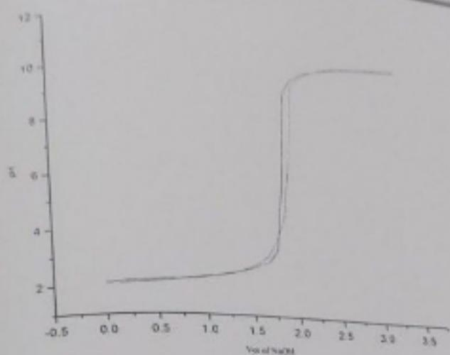
Graph 1.3 pH metric titration curve for Zn (II) + Nicotinic Acid (1:1 ratio)
