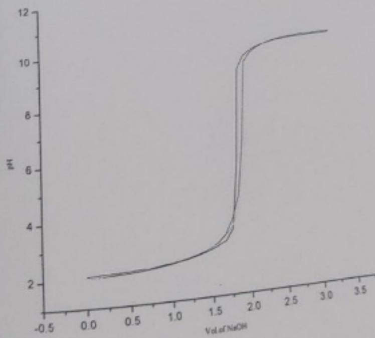
Graph 1.6 pH metric titration curve for Cd (II) + Nicotinic Acid (1:1 ratio)
