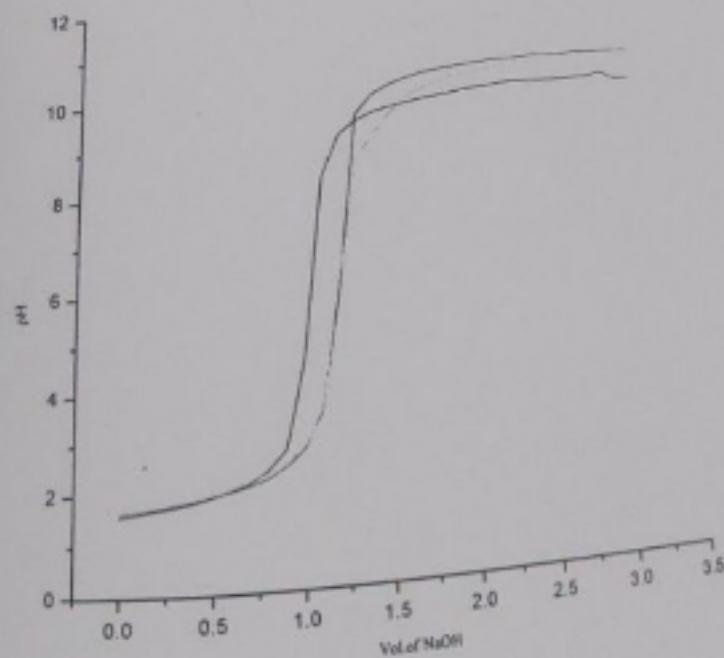
Graph 6.5 Potentiometric titration curve for Cd (II) + BPD (1:1 ratio)
