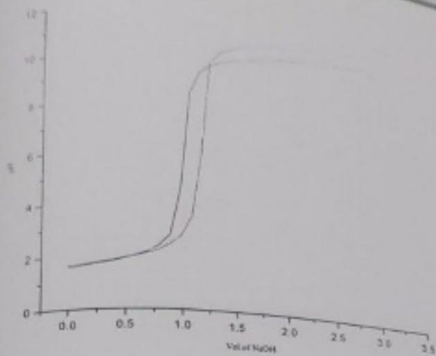
Graph 6.4 Potentiometric titration curve for Zn (II) + BPD (1:1 ratio)
