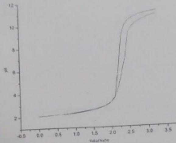
Graph 3.9 Potentiometric titration curve for Zn (II) + PABA (1:1 ratio)
