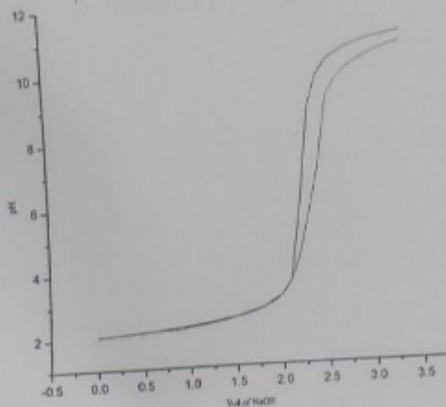
Graph 4.4 Potentiometric titration curve for Ni (II) + PABA (1:1 ratio)
