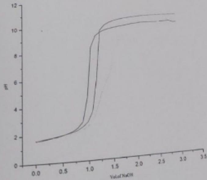
Graph 6.3 Potentiometric titration curve for Fe (III) + BPD (1:1 ratio)
