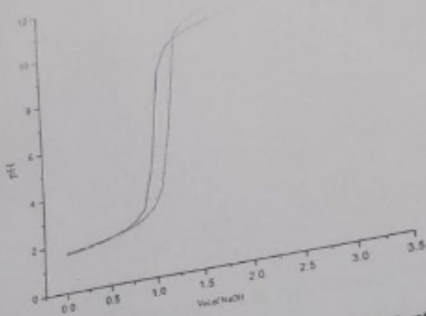
Graph 6.0 Potentiometric titration curve for Co (II) + BPD (1:1 ratio)
