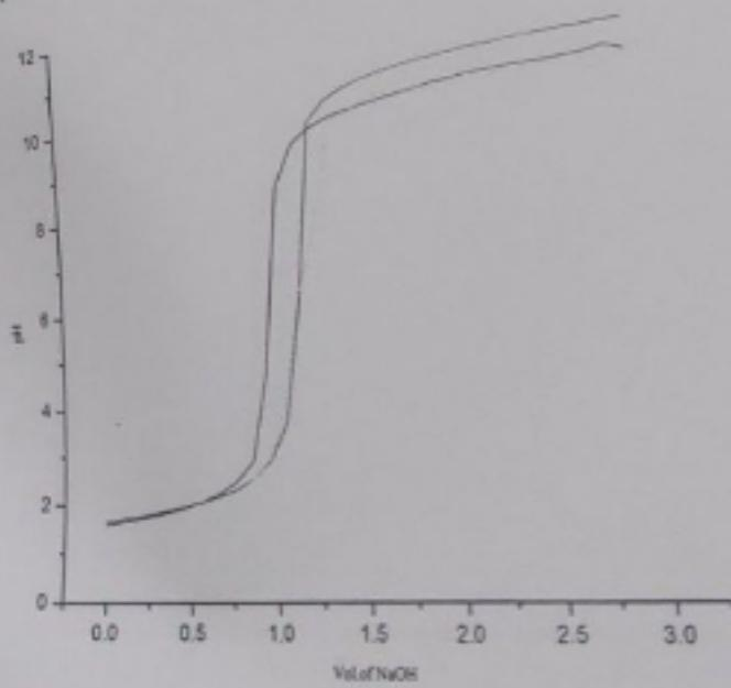
Graph 6.1 Potentiometric titration curve for Ni (III) +BPD (1:1 ratio)
