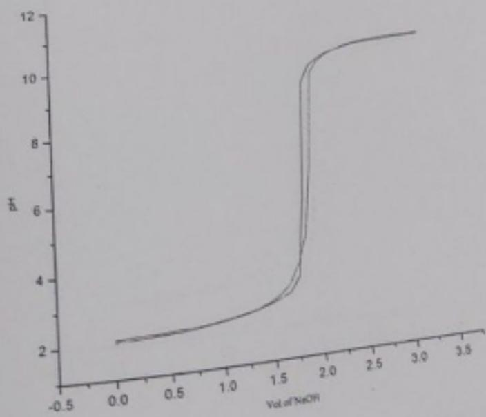
Graph 1.4 pH metric titration curve for Fe (III) + Nicotinic Acid (1:1 ratio)
