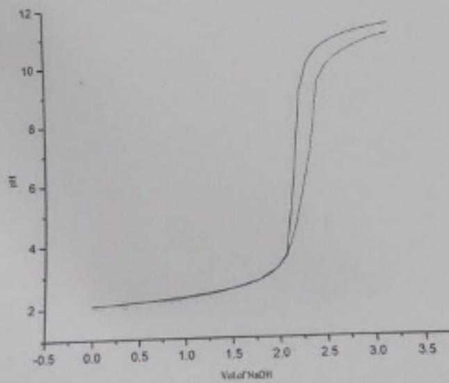
Graph 4.2 Potentiometric titration curve for Fe (III) + PABA (1:1 ratio)
